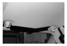
Tighten the screws on the visor arm to hold the visor bracket and light in place.
