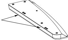
Place your bracket over the holes as pictured below and re-install the screws using the enclosed #8 washers (P30073-4) between the head of the screw and the bracket. Do this for both halves of the light, ensuring the brackets are mounted with the forks towards the outer edge of the light.
